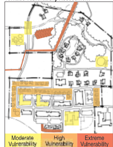
Tornado Vulnerability Assessment
