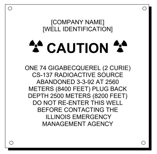
The size of the plaque should be convenient for use on active or inactive wells, e.g., a 17-centimeter (7-inch) square and 3 mm (1/8 inch) thick. Letter size of the word "CAUTION" should be approximately twice the letter size of the rest of the information, e.g., 12-millimeter (1/2-inch) and 6-millimeter (1/4-inch) letter size, respectively. Quantities and distances may be expressed either in SI units or in special and English units or in dual units.
